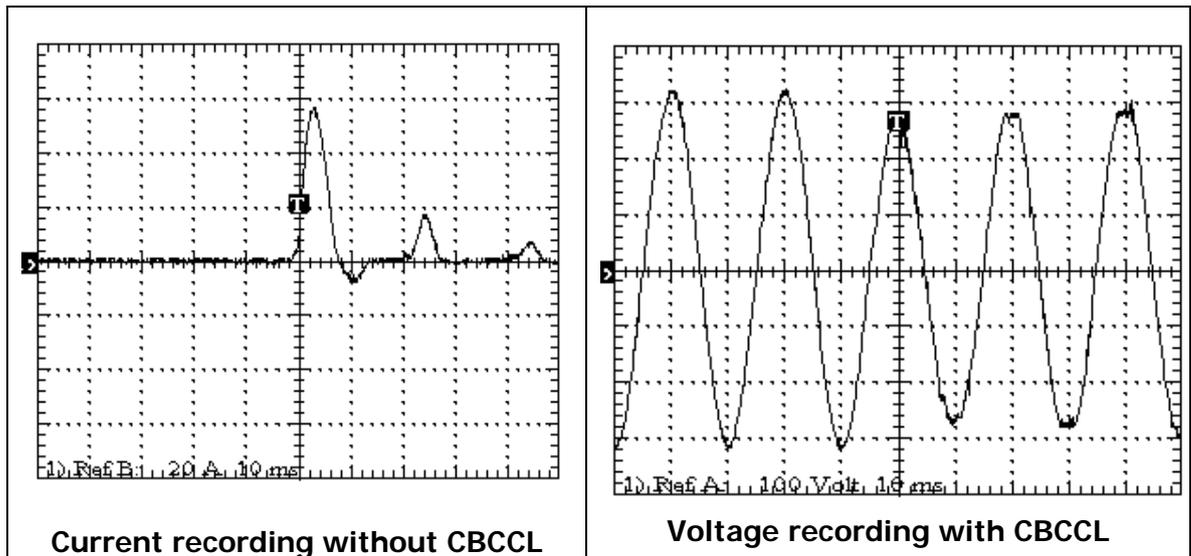
The recording below shows how the current limiting crawls up the sine wave acting at 30 kHz.
